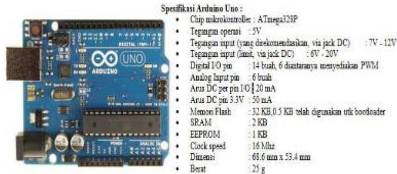
Gambar 1. Board arduino Uno R3
